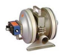
The Guardian rupture protection system can be fitted to all Flotronic Pumps. With this system a secondary chamber is created by an additional diaphragm behind each of the primary pump diaphragms to capture liquid upon primary diaphragm rupture. This chamber can be in low-cost Polypropylene (upgrade \*) or a material to match the pump wetted body (upgrade B).
