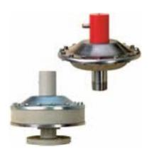
Dampers can be supplied integrally mounted on an FPL pump, as on the water-jacketed pump above, or individually to remove up to 95% of a given pulse on normal air supply pressure with no charging necessary. Dampers are provided in stainless steel, virgin or anti-static PTFE, PVDF, Polypropylene, aluminium or exotic materials with virgin or anti-static PTFE diaphragms as standard.
